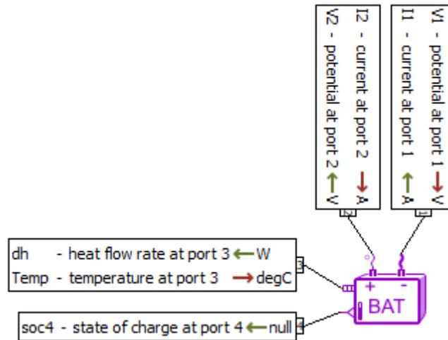
**Figure 5: Example of battery pack I/O (submodel ESSBATPA01)**
