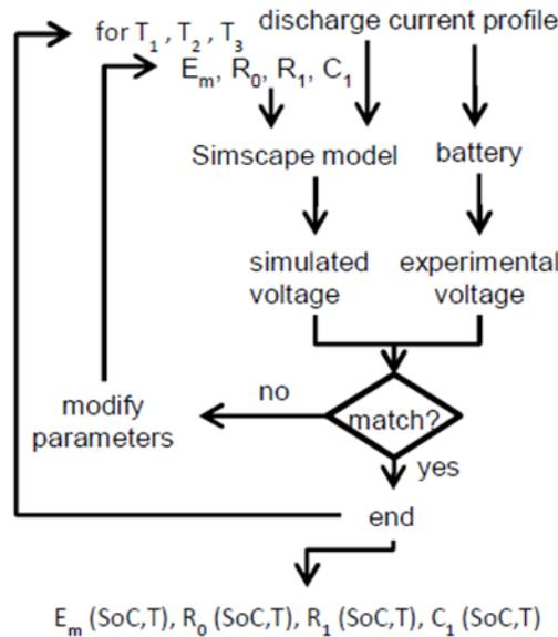
Figure 9: Flow diagram of the parameter's estimation procedure
