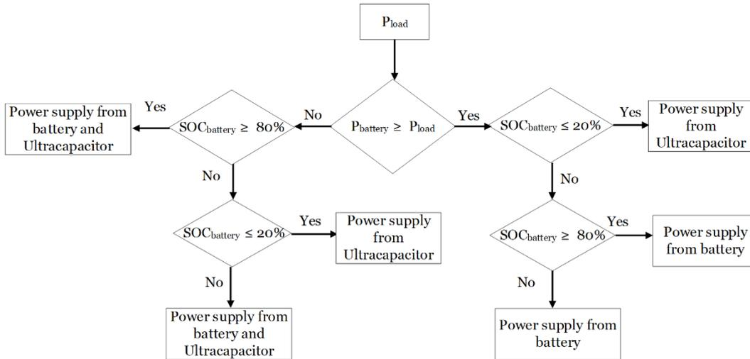
**Figure 18: Control algorithm for shaving peak-load demand with hybrid energy storage systems**
