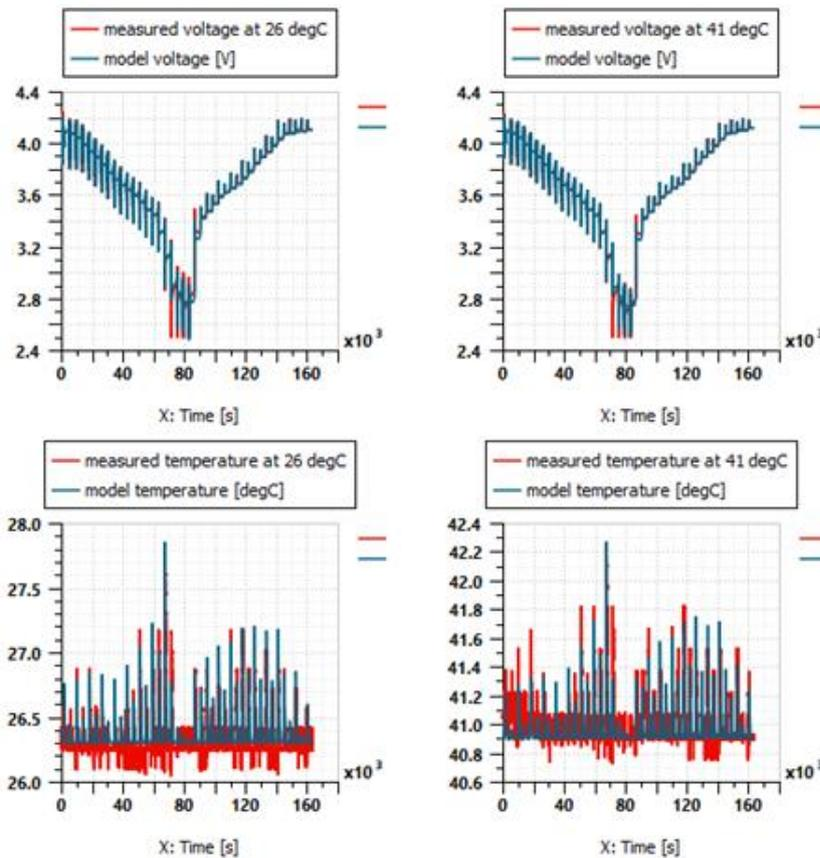
Figure 10: Voltage and temperature comparison between the experimental and model data for hybrid pulse tests at different temperatures
