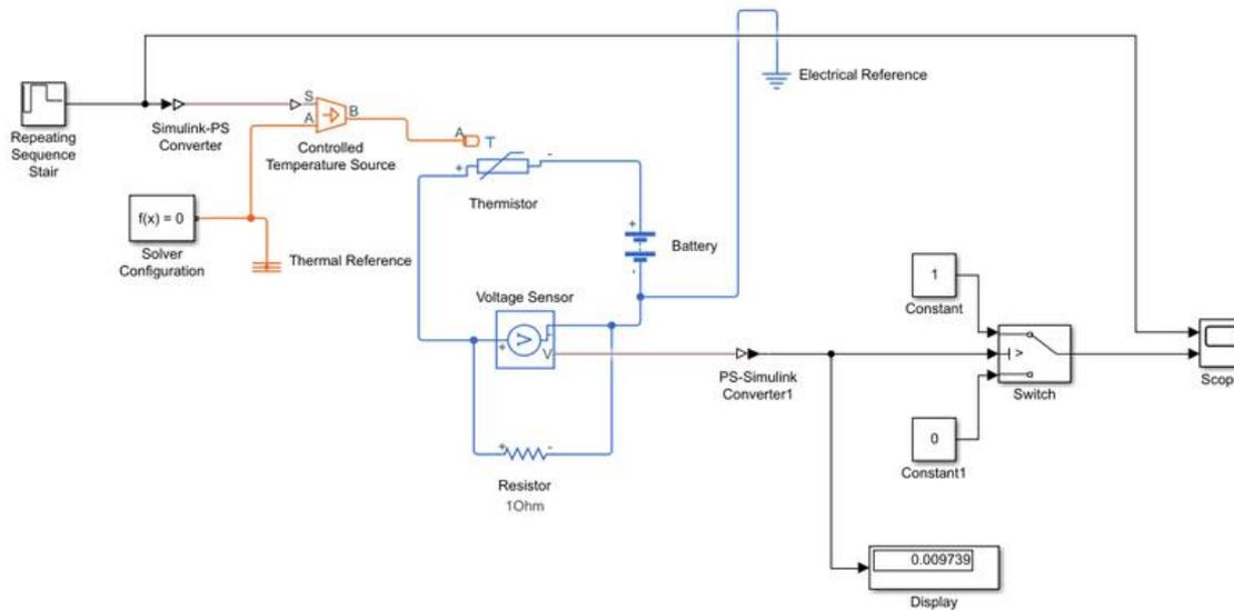
**Figure 3: Connecting Simscape diagrams to Simulink sources and scopes**
