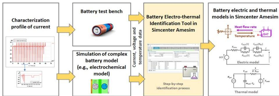
Figure 8: Workflow of the battery electro-thermal identification tool
