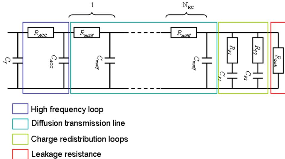
**Figure 15: Dynamic UCAP phenomena modelled with an equivalent electrical circuit**
