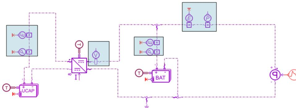
**Figure 19: Example of plant model of a hybrid storage system with additional sensor for PMS/EMS connection**
