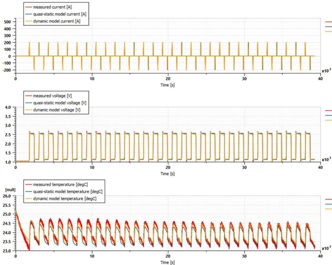
**Figure 16: Comparison between experimental and modelling voltages and temperatures**
