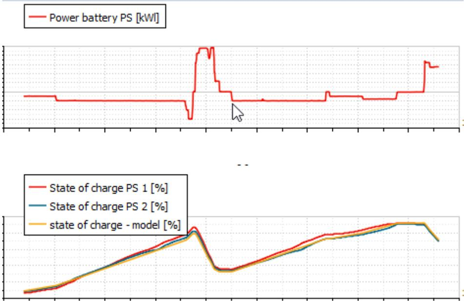
Figure 26: Simcenter Amesim results: power demand on the battery pack and state of charge comparison of the model with recorded state of charge measurements
