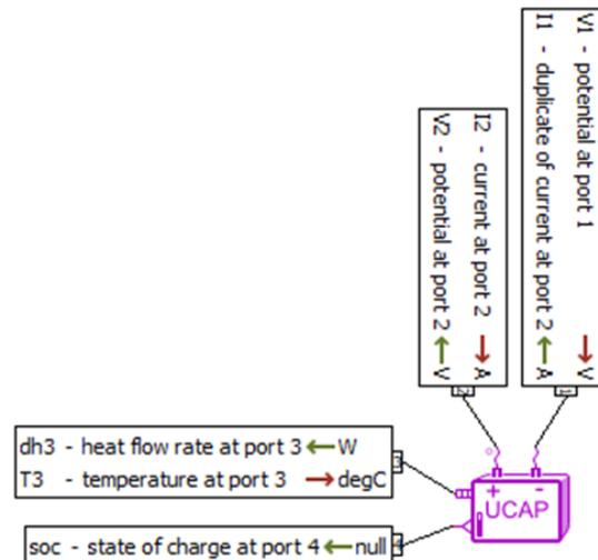
**Figure 13: Example of supercapacitor pack I/O (submodel ESSUCAPPS01)**
