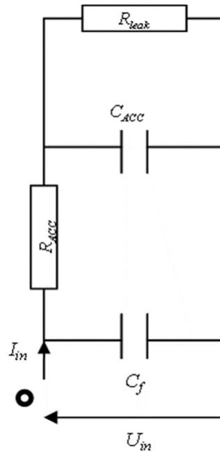
**Figure 14: Electrical equivalent circuit model of the quasi-static UCAP submodel**
