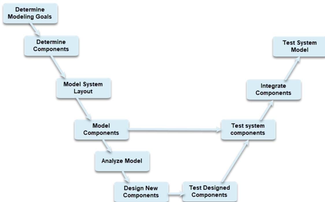
Figure 2: Model-based design task considering the workflow
