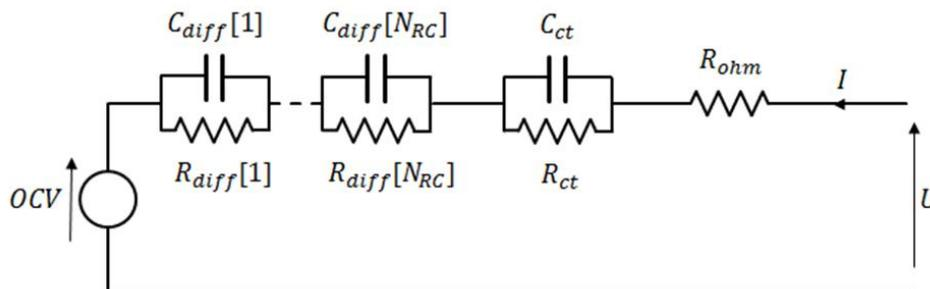
**Figure 6: Dynamic equivalent circuit model of battery cell**
