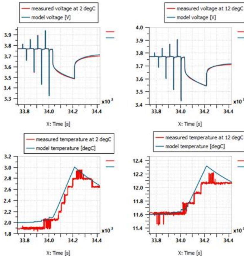
**Figure 11: Zooms of the results for the hybrid pulse tests**
