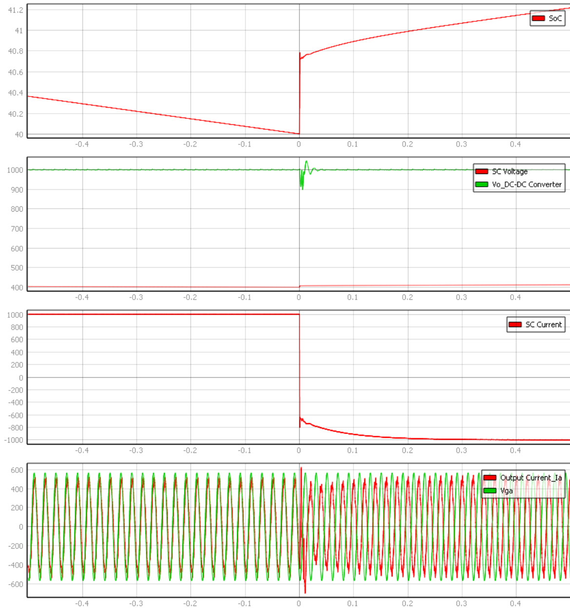
Figure 66: Discharging/charging waveforms of SC at 1000A
