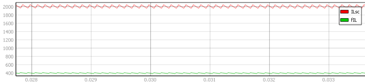
Figure 71: SC and SSB current waveform ( I_{ref\_SC} = 2000A , I_{ref\_SSB} = 400A )
