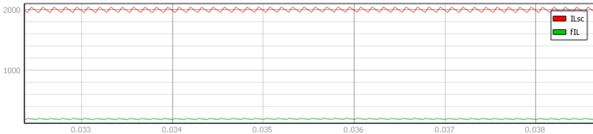
Figure 69: SC and SSB current waveform ( I_{ref\_SC} = 2000A , I_{ref\_SSB} = 200A )
